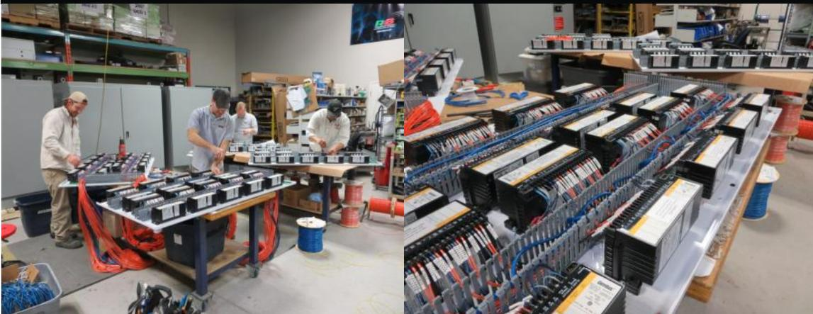
Our fellows in the Mississauga Panel Shop are working on multiple boards of programmable controllers which are being pre-fabricated and installed in cabinets. This method allows for everything to go through strict quality control and testing processes in a clean and dry environment.
